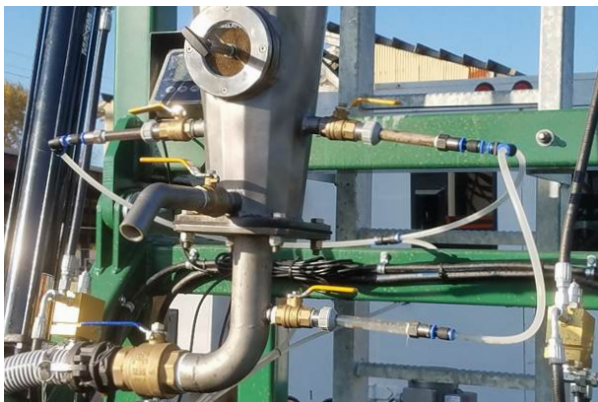
Figure 3. Struvite recovery point from the cone fluidized bed system.
