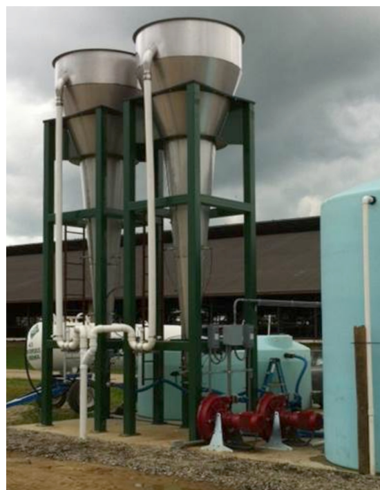
Figure 2. Cone fluidized bed system for struvite recovery.
