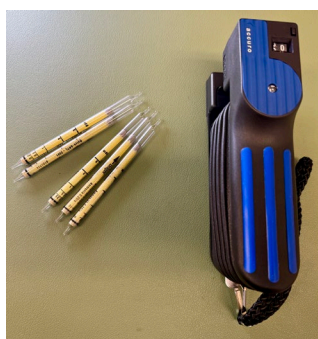
Figure 3. Colorimetric ammonia detection tubes and a piston hand pump (photo: Nesli Akdeniz)
